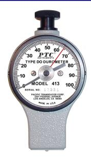
ASTM Type DO measures the indentation hardness of Fireproof Coating, Paint, Moderately Hard Rubber, Elastomers and Dense Textile Windings.
